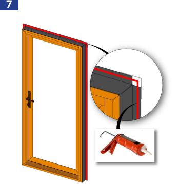
Apply a continuous 3/8" bead of sealant around the interior side of the position fin.
