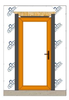
Cut two pieces of flashing tape for jamb flashing extending 1" above the head position fin. Apply flashing tape and smooth using J-roller.
