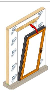
Center the door in rough opening, lifting and setting the bottom of the door in first, then tilting into place.. Verify for e out of sealant all along position fin.
