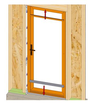
Install the jamb covers, then the head cover and threshold.
